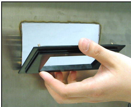
Figure 17: Installation de la plaque adaptatrice
