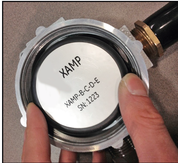
Figure 22: Junction Box Cap
