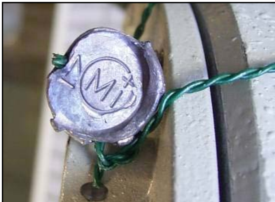
Figure 42: NMI Lead Seal - Typical
