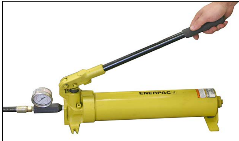
Figure 81: Pressurizing the Hydraulic Pump
