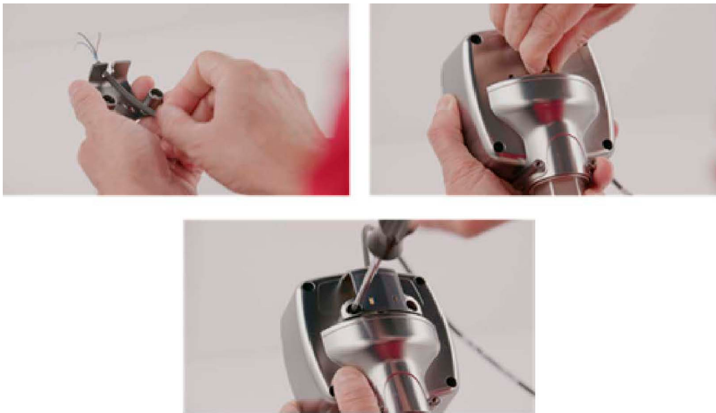
Figure 4: HygroPro II installation step 1 – initial wiring
