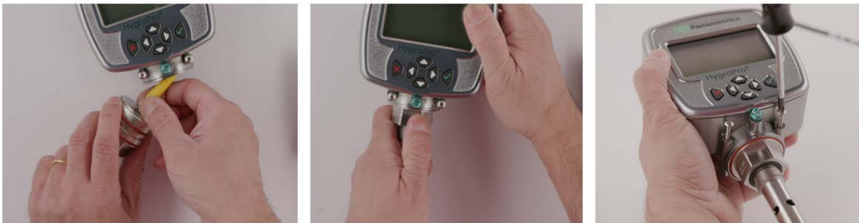
Figure 19: Reinstalling the HygroPro II RTE probe into the dismantled transmitter
