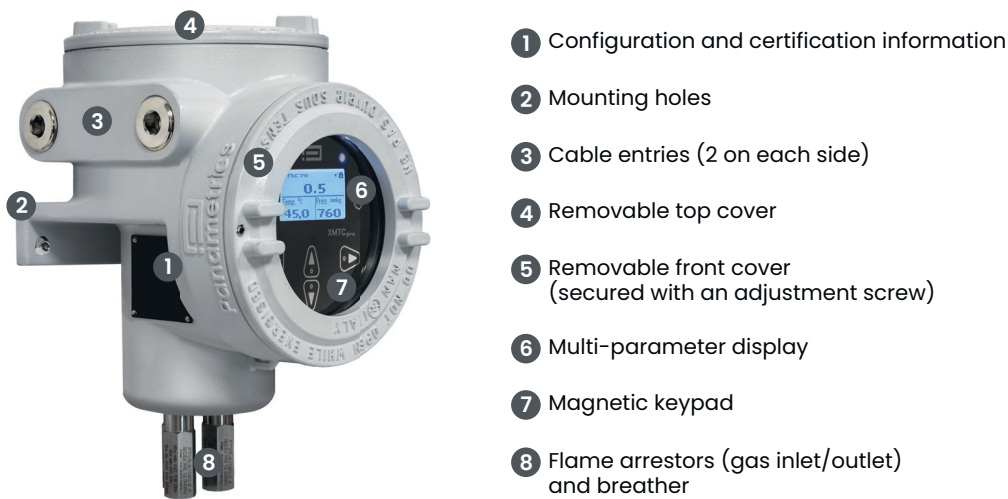
Figure 1: External Components of the XMTCpro
