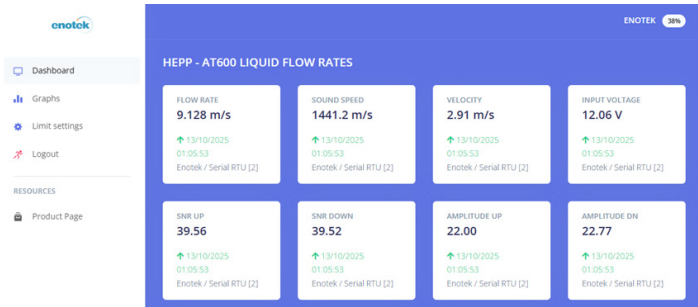
AT600 flow and diagnostics data
