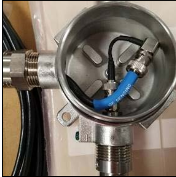
Figure 17: Transducer Cable Connection with Cable Jumper, PN133M7313-03
