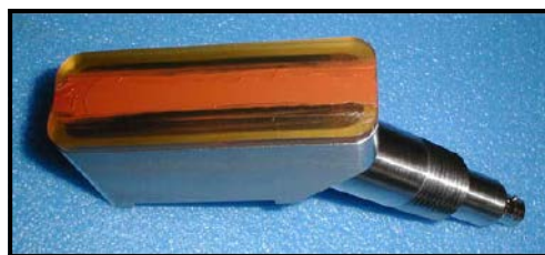
Figure 25: Couplant on Transducer Face
