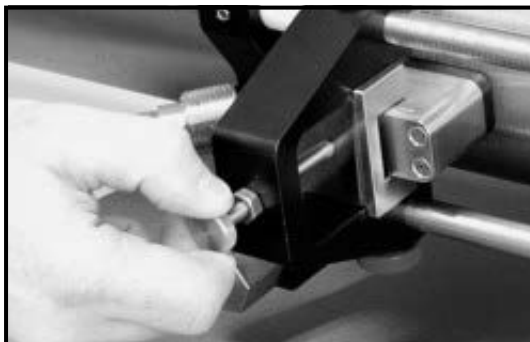
Figure 26: Installing the First Transducer
