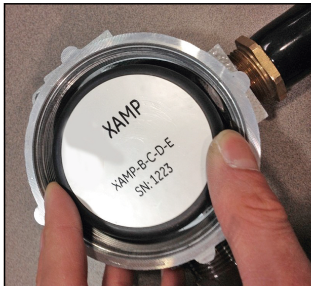
Figure 12: Junction Box Cap
