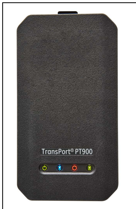
Figure 49: Battery Charging Status LEDs
