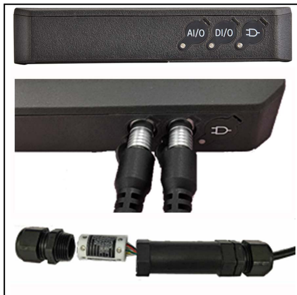
Figure 46: Transmitter I/O Connections (Right Side)
