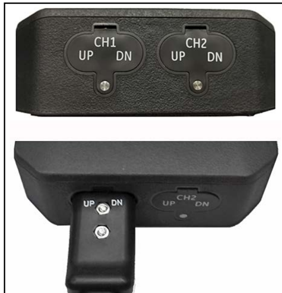
Figure 45: Transducer Connections (Bottom)
