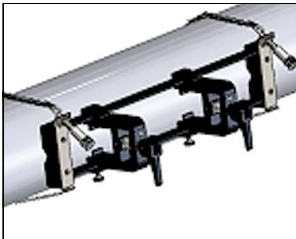
Figure 15: Fixture With Chains Installed
