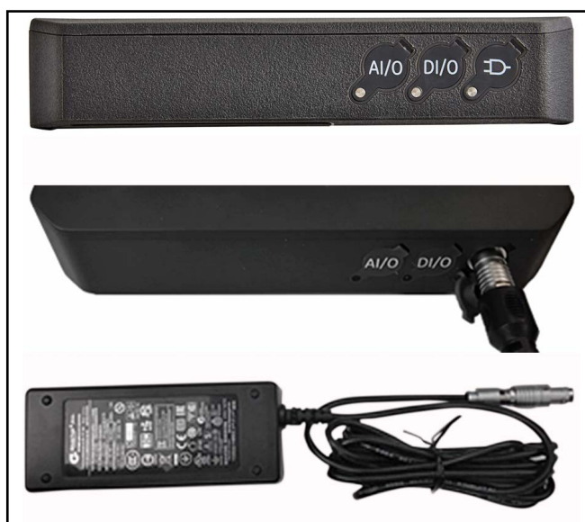
Figure 44: Transmitter Power Connection (Right Side)
