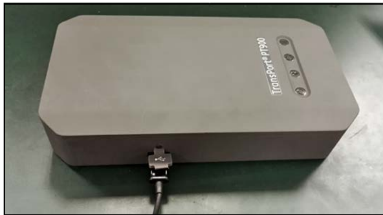
Figure 118: USB Cable Connected to the Transmitter
