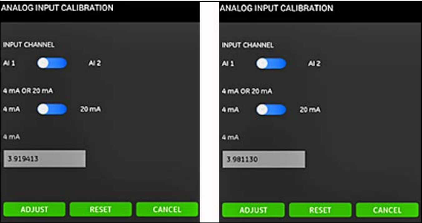
Figure 127: Before (Left) and After (Right) 4 mA Values
