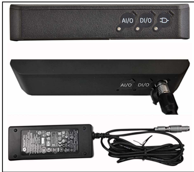
Figure 44: Transmitter Power Connection (Right Side)
