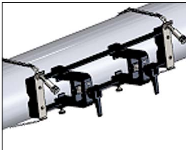
Figure 15: Fixture With Chains Installed
