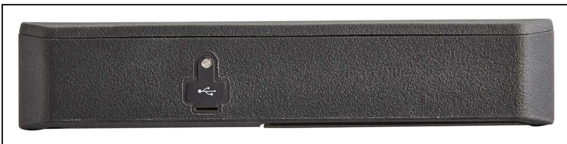
Figure 48: Transmitter USB Connector (Left Side)
