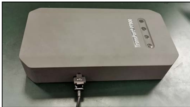
Figure 119: USB Cable Connected to the Transmitter
