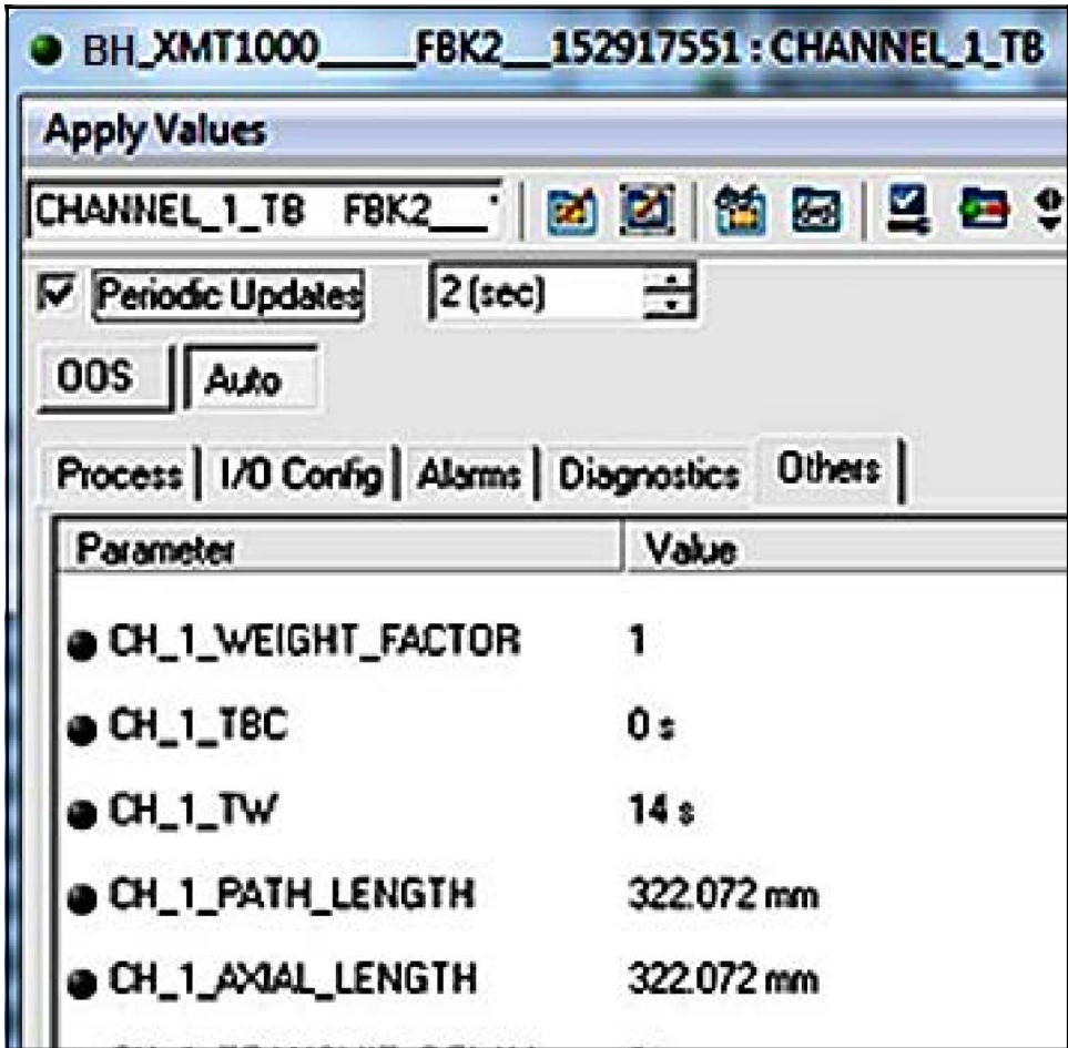
Figure 75: Channel Transducer Block
