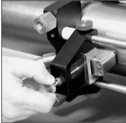
Figure 20: Installing the First Transducer
