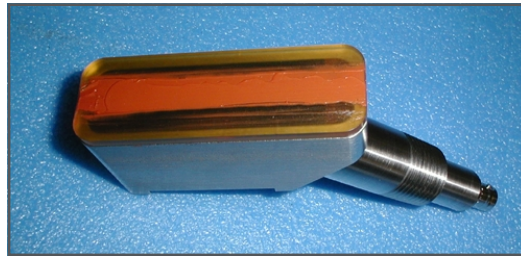
Figure 31: Couplant on Transducer Face
