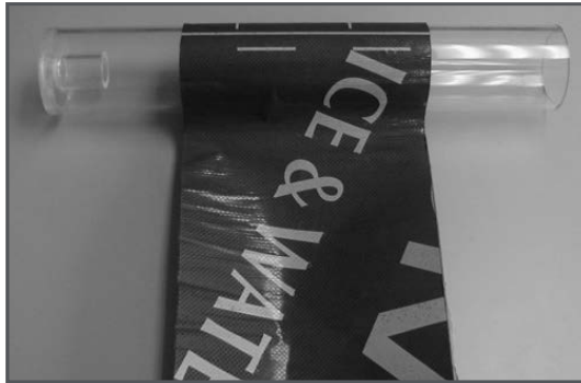
Figure 32: DMP-1 Dampening Material Wrapped Around Pipe
