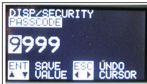
Figure 42: Security check window
