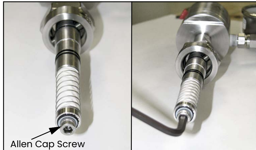
Figure 16: Checking/Tightening the Allen Cap Screw
