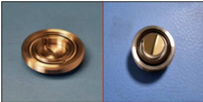
Figure 97: Replacing Cleaned Mirror into End Cap Assembly
