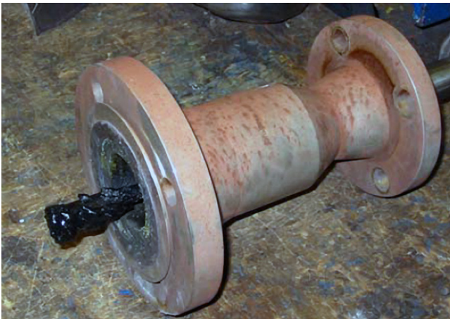
Fig. 4: Upstream transducer removed for inspection
