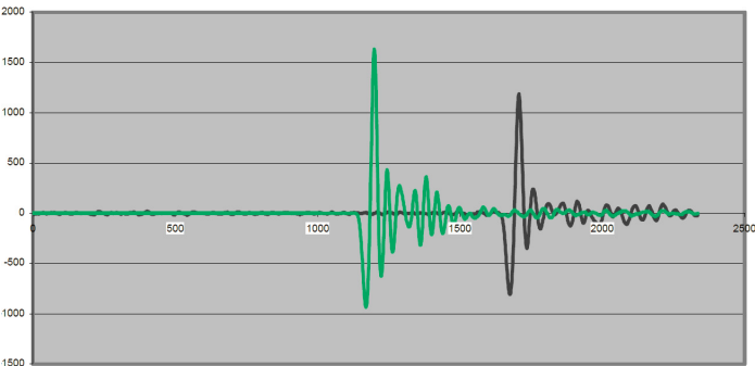
Fig. 3: Ultrasonic signal from GM868 installed on 80 in. (2000 mm) pipe
