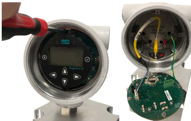
Figure 8: HygroPro XP installation step 4 - unfasten the HMI
