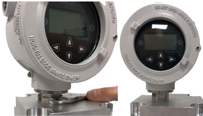
Figure 6: HygroPro XP installation step 2 - installing into sample cell
