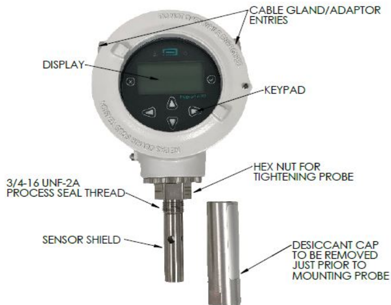
Figure 4: Key HygroPro XP parts relevant to installation
