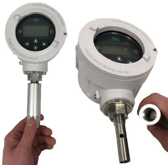
Figure 5: HygroPro XP installation step 1 - removing desiccant cap
