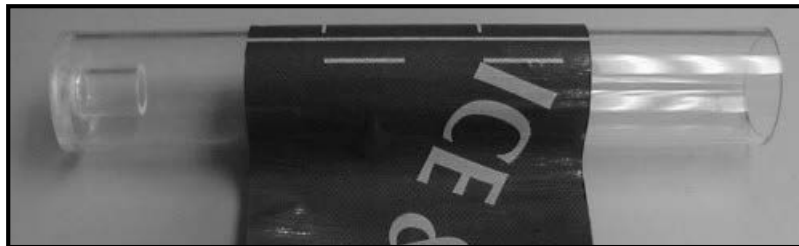
Figure 22: DMP-1 Damping Material Wrapped Around Pipe
