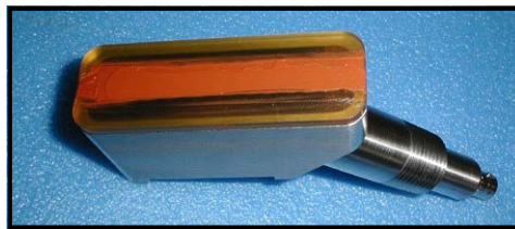
Figure 9: Couplant on Transducer Face
