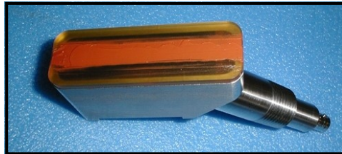
Figure 21: Couplant on Transducer Face
