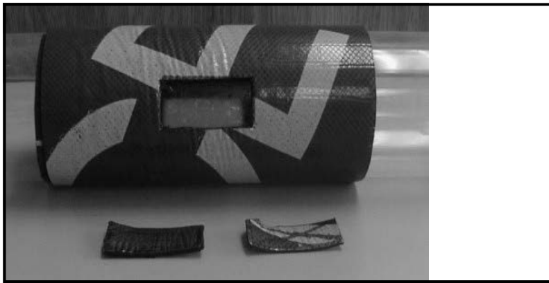
Figure 24: DMP-1 Material with Transducer Footprint Cut Out
