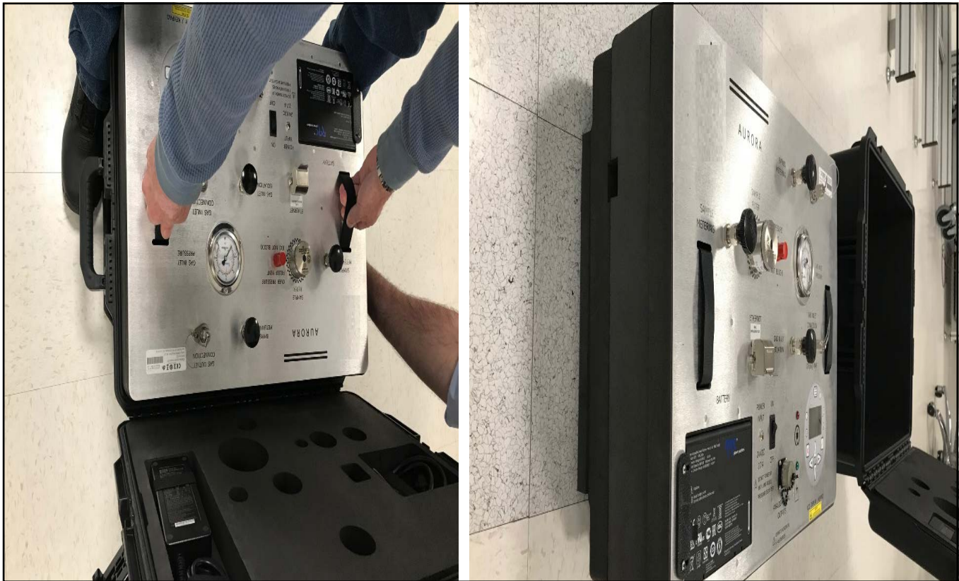
Figure 52: Extraction of Inner Foam Assembly from TransPort Pelican Case for Access to Absorption Cell End Mirror
