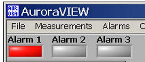
Figure 33: Alarm Status Indicators
