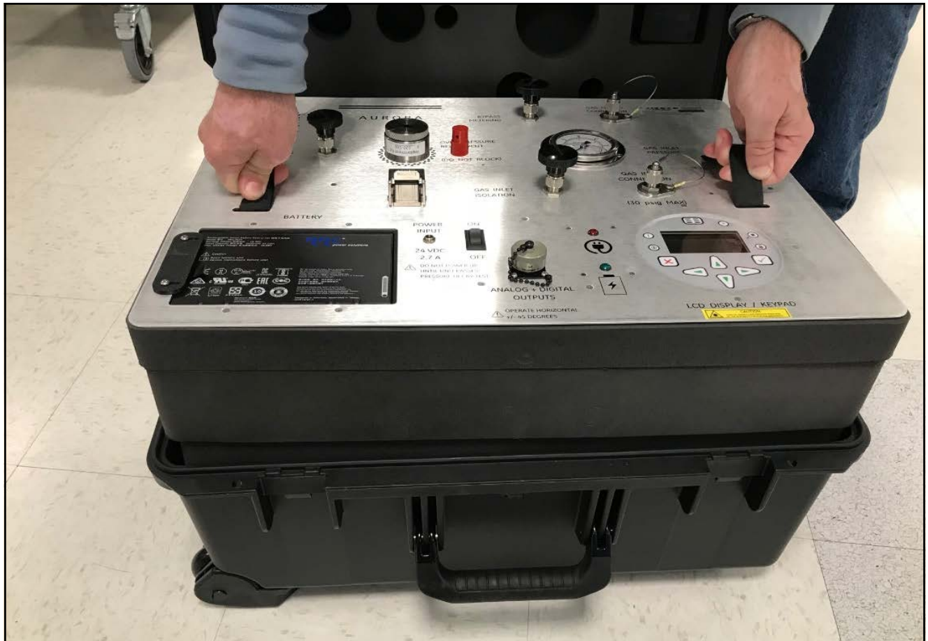
Figure 60: Replacing Inner Foam Housing into the External Pelican Case After Mirror Cleaning
