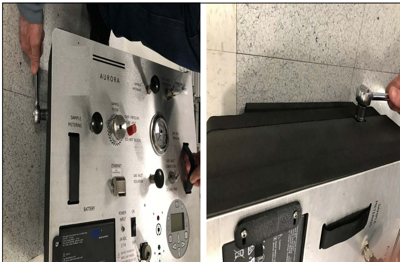
Figure 53: Extraction of Absorption Cell End Mirror from Inner Foam Housing while Holding the Assembly Upright to Prevent the Mirror from Falling out
