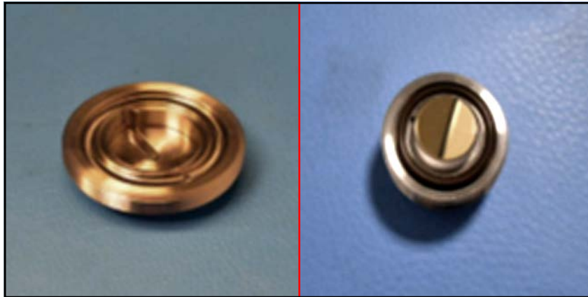
Figure 58: Replacing Cleaned Mirror into End Cap Assembly
