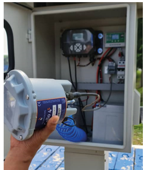
Fig. 1: Cabinet with AT600 electronics, data logger, battery and 4G communication module
