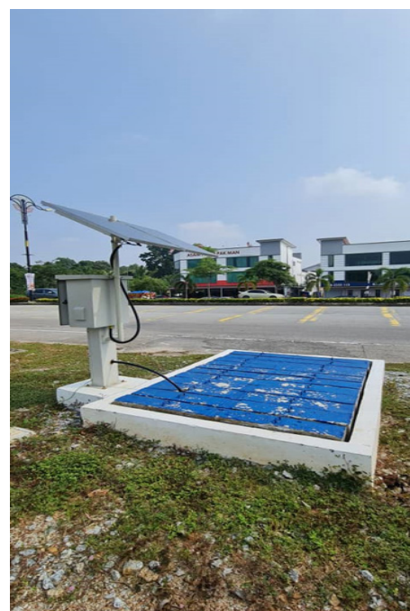
Fig. 2: Solar panel powering the AT600 battery in the cabinet which connects to the IP68 C-RS 401 transducers underground
