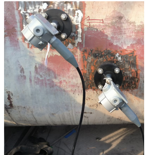
T5 Bias 90 installation with XAMP preamplifiers on the 64" (DN1600) line
