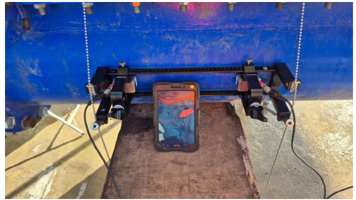
Fig. 2: PT900 on the robot insertion mechanism (DN350)
