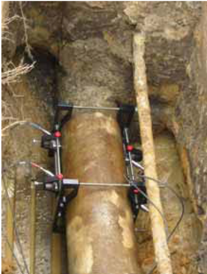
C-RL-304 transducers installed on a 12 in (300 mm) asbestos cement pipe downstream of reducing station
