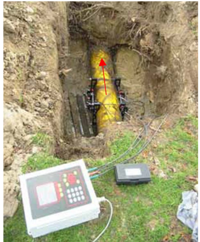
C-RL-304 Transducers installed on a 12 in. (300 mm) PVC pipe downstream of reducing station
