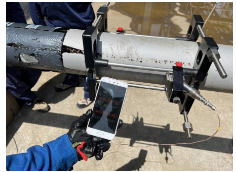
Fig. 1: Clamp on installation on high pressure hydrogen line
