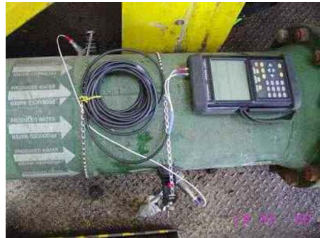
PT878 in use on 12-inch Produced Water line, with insertion-turbine 3D downstream
