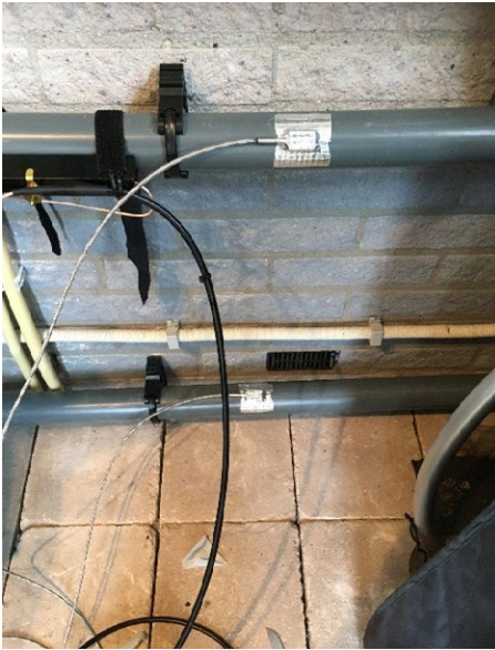
PT1000 elements (on inlet and outlet) and small clamping fixture
